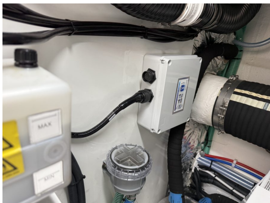
Controller mounted with the Y-tap HDP20 plug connected and locked.
