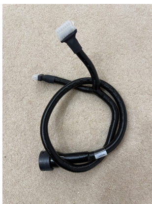
The Y-tap cable: two Mini-Fit Jr ends and one HDP20 controller plug.
